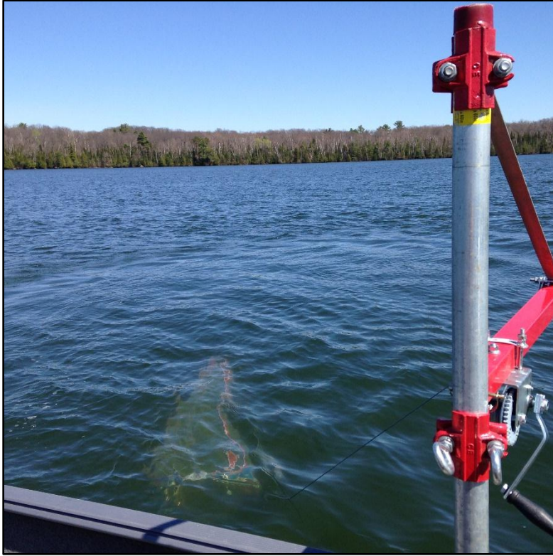
FIGURE 2 – Custom-made boom used to tow ichthyoplankton nets at shallow (1.0-1.5 m) and deep (2.0-2.5 m) depth ranges. The boom extended perpendicularly over the hull of the boat. A steel cable extended from the reel on the boom and was clipped to the bridle of the net. Downrigger balls (approximately 4 kg) were attached to the frame of the net, and the cable was extended until the net reached desired depth range.
