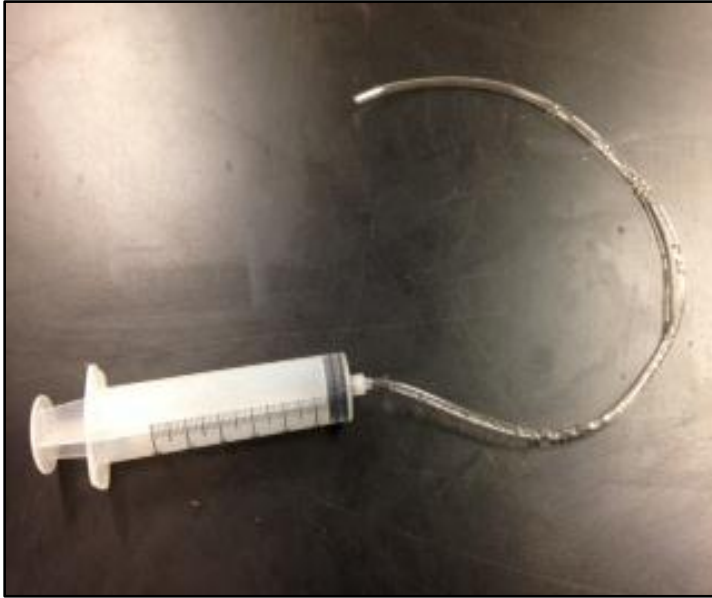
FIGURE 4 – Small gastric lavage used to remove diet contents of panfish and other small (> 200 mm TL) fish that might prey upon larval walleyes. The gastric lavage consisted of a livestock syringe fitted with small plastic tubing (0.16-cm diameter). The syringe was filled with water and the tube inserted through the mouth and into the esophagus. Fish were turned upside down over a mesh-lined funnel as diet contents were flushed out. Fish were released and diet items preserved for further analysis.
