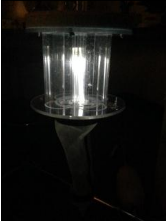
FIGURE 3 – Plexiglas quatrefoil light trap used to sample larval fish in 2014. Light traps were illuminated by a battery powered LED light, with four 4-mm slots at points of the cloverleaf configuration through which larvae enter. Traps were anchored using a small concrete anchor, and Styrofoam floats fixed to the top of the traps ensured the traps floated just below the water surface. A 1,000- \mu m mesh conical net was attached to the bottom of the light trap where larvae were entrapped.
